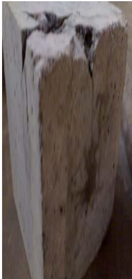
Figure 4.6 crack pattern in Cube
